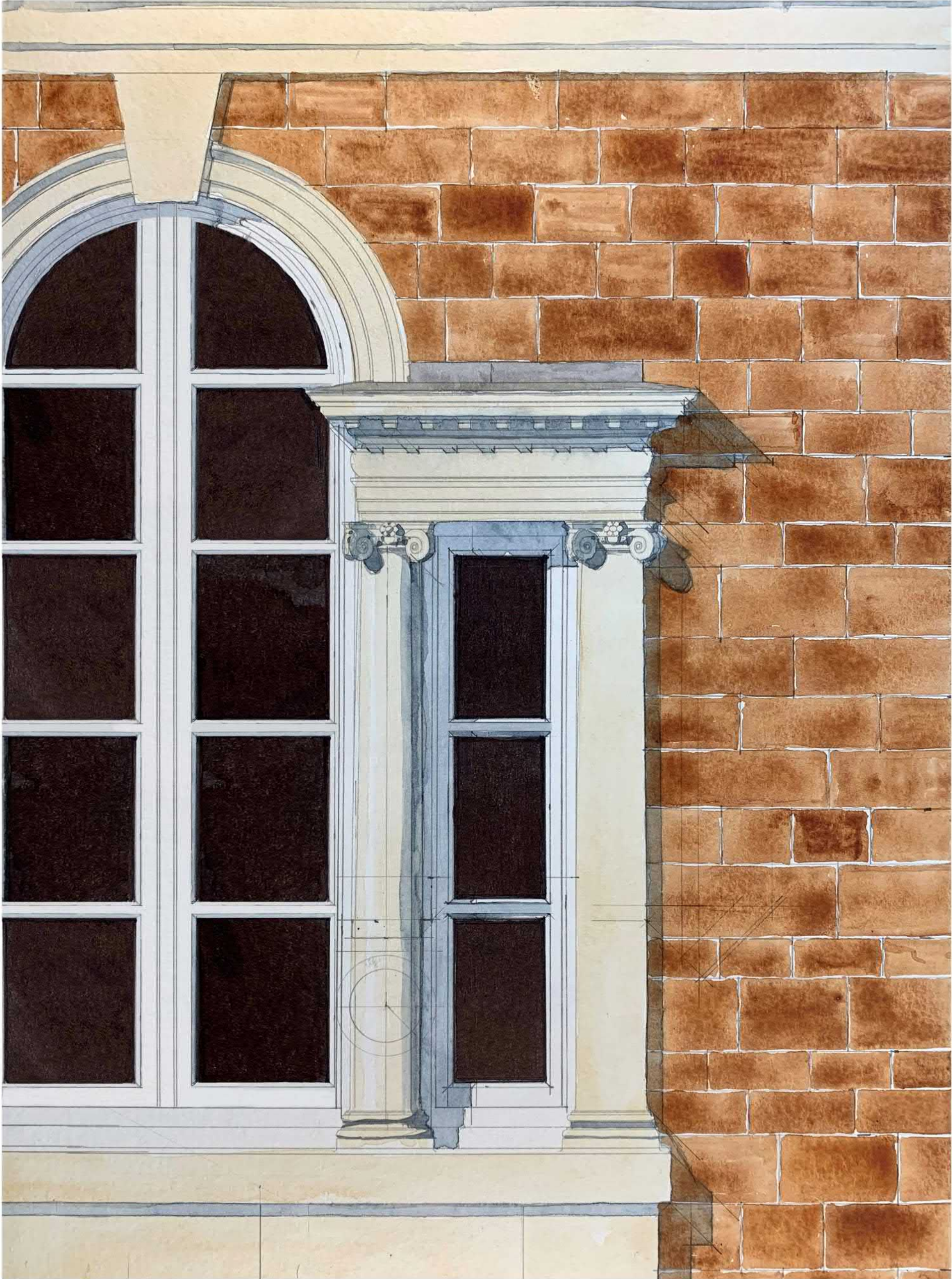
ELEVATION SHOWING VENETIAN WINDOW
